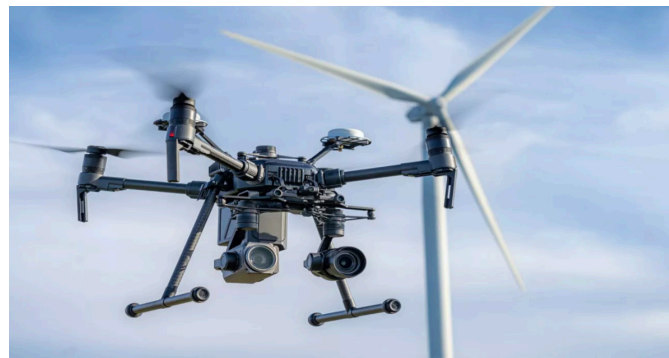
Drones are now being used to inspect wind farm blades
