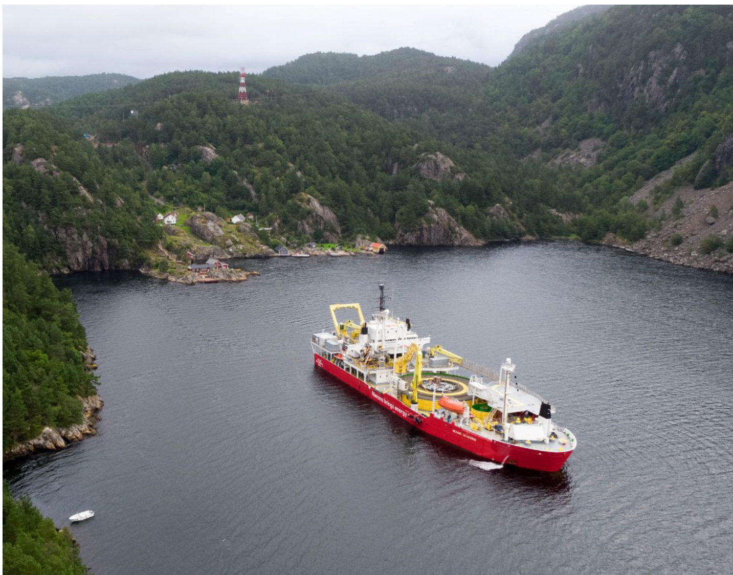
A vessel lays the first meters of the NordLink subsea cable in Summer 2017 Source: TenneT
