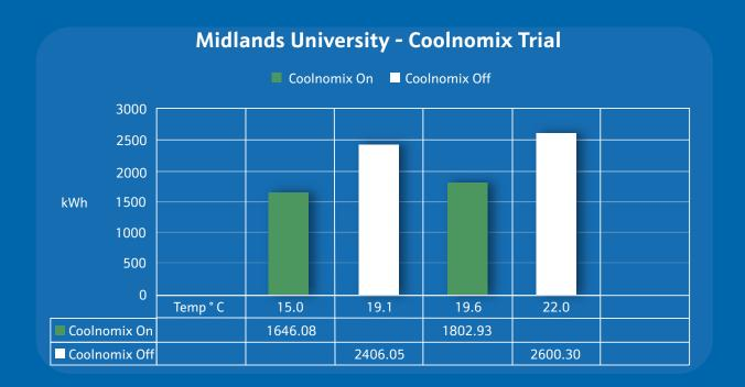
This is clearly shown, when comparing similar outside temperatures, the graph shows that when COOLNOMIX is not connected the air-conditioning unit was using 33.5% more energy than when COOLNOMIX is connected and operating.
